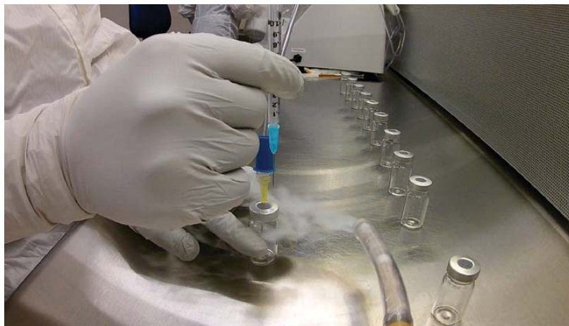
Figure 4. After risk mitigation, unidirectional airflow without turbulence sweeps over and away from the critical site.
