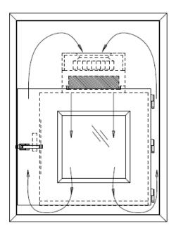
1) The pass through has HEPA filtration introduced at the ceiling of the pass-through.
