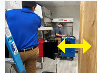
How the obstruction was used to simulate various distances between the front intake opening and a wall. The yellow arrow represents where the corresponding distance was measured.
